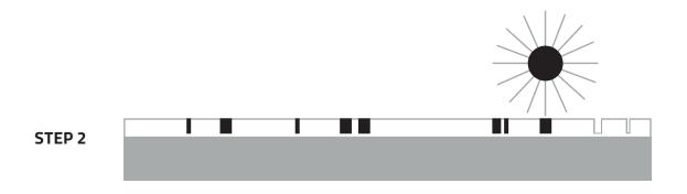
The printed texture is softer than the wear layer. The texture is removed by mechanical means.
