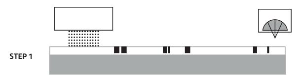
The texture is digitally printed into the wear layer. Texture and wear layer are cured.
